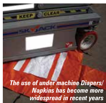
The MEC LCS leak containment system
