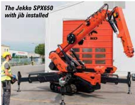
As you might expect it incorporates all of the innovations from those two machines and more. It is powered by a custom designed and built 48 volt lithium-ion battery pack, with on board charger, which takes nine hours to recharge on a domestic 230 volt plug, but the crane can also work while it is being recharged. Charging with a remote 400 volt high power charger takes only three hours from empty to full.
