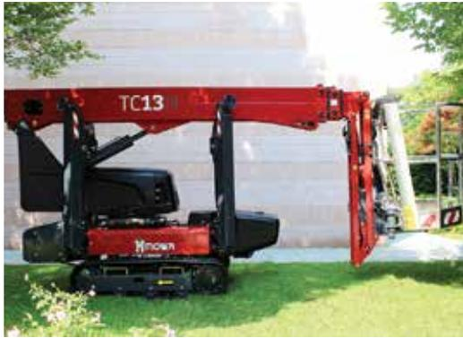
The lift has an overall length with basket removed of just under 3.7 metres, an overall width of 748mm and an overall height of just under 1.95 metres. The extended outrigger footprint is 2.45 by 2.9 metres.
