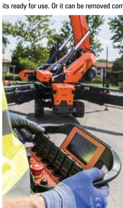
The machine's overall stowed width is 988mm, but the tracks extend hydraulically to 1.38 metres for greater stability on site.
