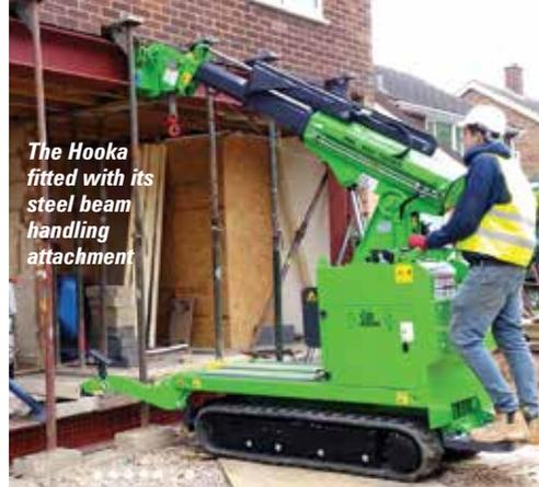
The Hooka fitted with its steel beam handling attachment
