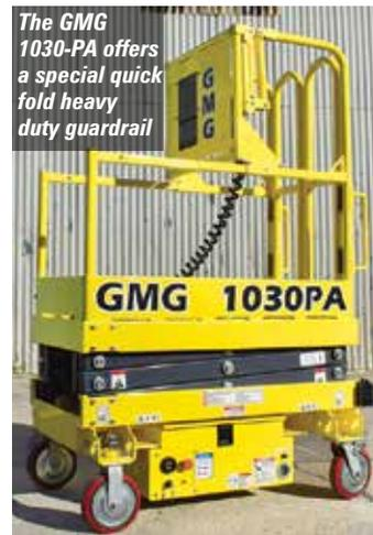
*The GMG 1030-PA offers a special quick fold heavy duty guardrail*
