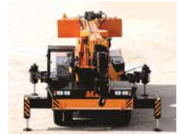
The addition of four outriggers allows it to double up as a 360 degree slewing crane.
