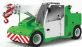
an overall length of 3.96 metres and at 1.97 metres overall height will pass under two metre overhead obstructions.
