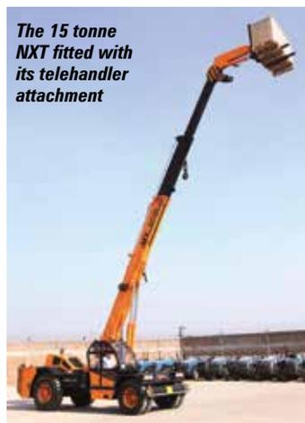
The 15 tonne NXT fitted with its telehandler attachment
