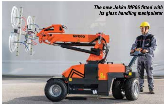
The new Jekko MP06 fitted with its glass handling manipulator
