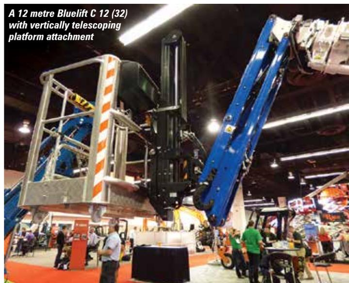
A 12 metre Bluelift C 12 (32) with vertically telescoping platform attachment
