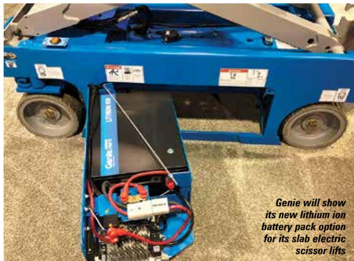
*Genie will show its new lithium ion battery pack option for its slab electric scissor lifts*
