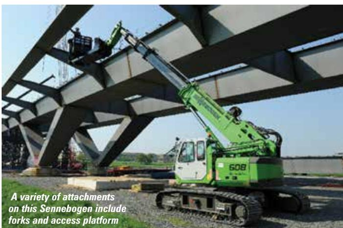
*A variety of attachments on this Sennebogen include forks and access platform*
