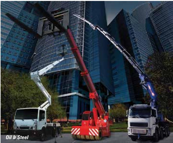
The telescopic MTE 270 EX has a 250kg platform capacity. The rear outriggers of the platform remain permanently within the vehicle width, while the front outriggers can be set up in-line or extended on one or both sides. Even with the outriggers in-line the platform offers 16 metres of outreach over the rear and nine metres to the side. Extending the rear outriggers increases this to 13 metres. The MTE 270 EX is available mounted on a Mercedes Sprinter or on an Iveco Daily chassis.
