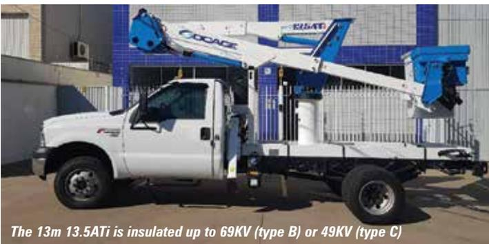
*The 13m 13.5ATi is insulated up to 69KV (type B) or 49KV (type C)*
