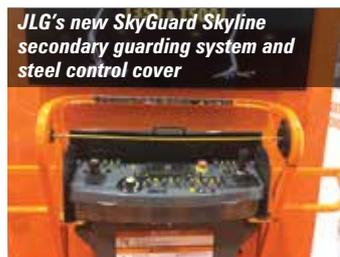
JLG's new SkyGuard SkyLine secondary guarding system and steel control cover
