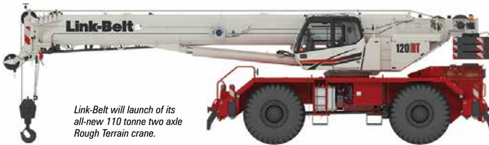
*Link-Belt will launch of its all-new 110 tonne two axle Rough Terrain crane.*
