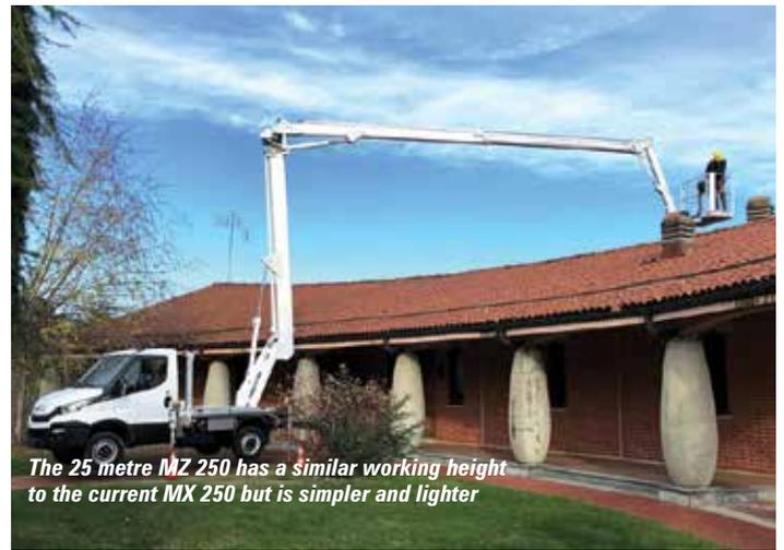
*The 25 metre MZ 250 has a similar working height to the current MX 250 but is simpler and lighter*
