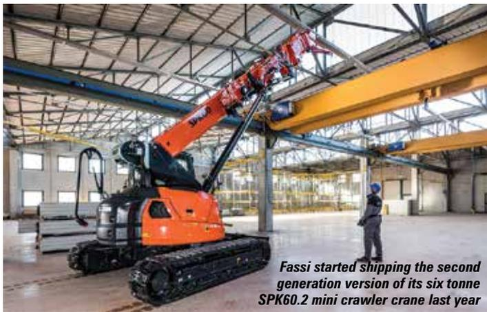
Fassi started shipping the second generation version of its six tonne SPK60.2 mini crawler crane last year
