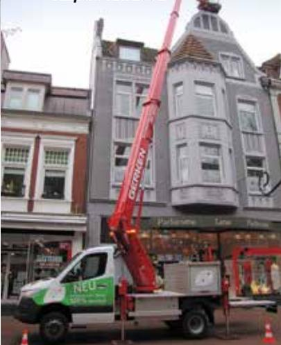
platform uses the chassis battery pack, which Ruthmann says is sufficient for a complete working day, including up to 100 km of driving and four hours continuous platform operation. The charging time at a 380 volt charging station is four hours, longer on conventional 230 volt sockets.
