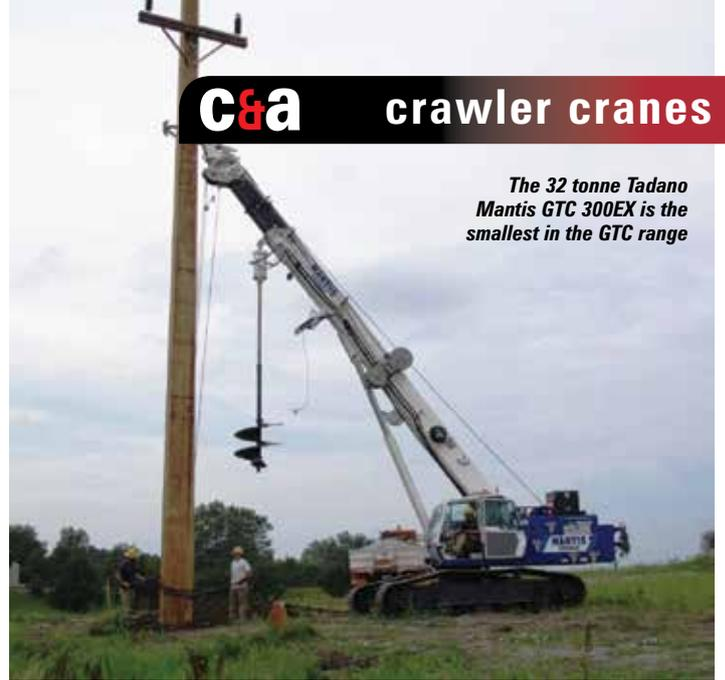
*The 32 tonne Tadano Mantis GTC 300EX is the smallest in the GTC range*
