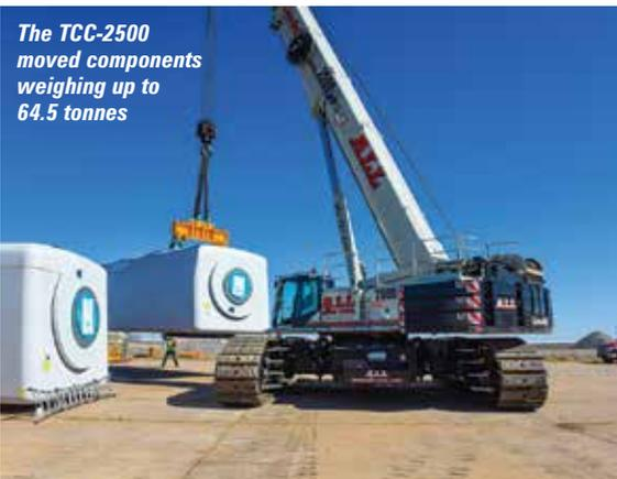
The TCC-2500 moved components weighing up to 64.5 tonnes
