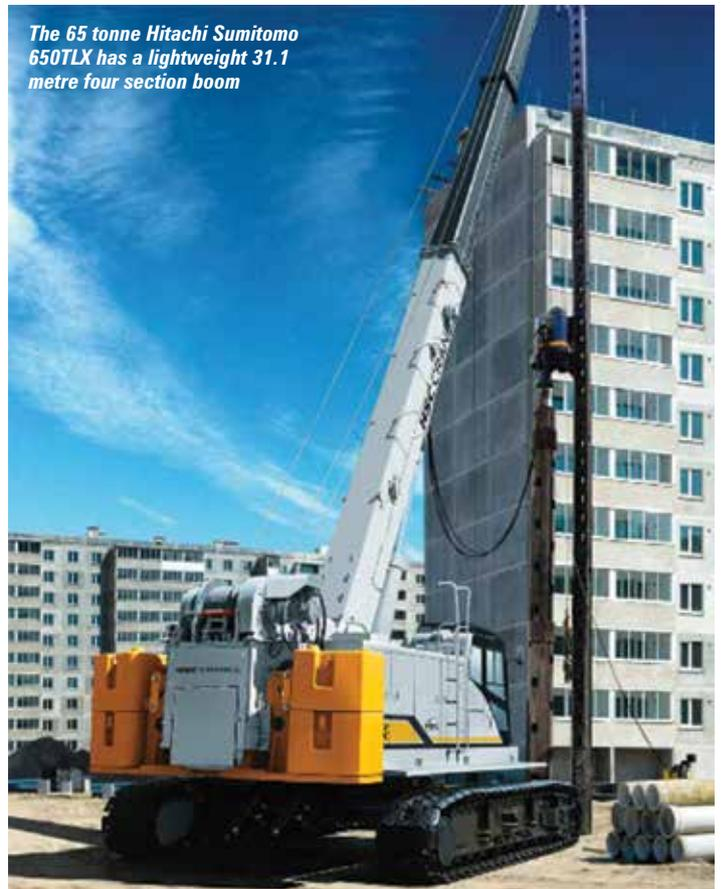
*The 65 tonne Hitachi Sumitomo 650TLX has a lightweight 31.1 metre four section boom*
