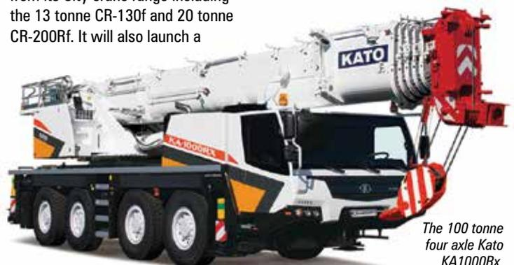
The 100 tonne four axle Kato KA1000Rx.
