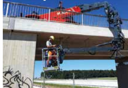
Fitted to Magni's RTH 5.21, the TP O-U can work up to 6.9 metres under the bridge deck
