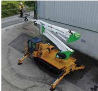
Features include a 250kg unrestricted platform capacity, 360 degree continuous slew, 180 degrees platform rotation and low pressure hydraulic controls. The Morooka MST800VDL diesel powered chassis features 595mm wide rubber tracks, has an overall width of 2.7 metres and four fold down outriggers. Overall weight of the machine is 10.3 tonnes and offers travel speed of up to 12kph.
