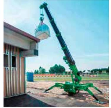
Weighing 2,300kg - or 2,740kg with the extension - the RPG 2900 has an overall stowed width of 730mm an overall height of 1.5 metres, and an overall length of just over three metres. It has classic spider type outriggers with three different positions to suit various space requirements, including a 90 degree configuration and narrow jacking.
