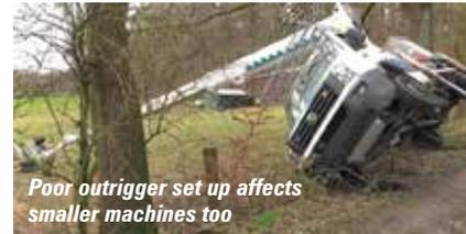
Poor outrigger set up affects smaller machines too
