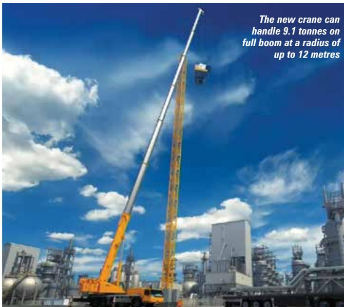
The new crane can handle 9.1 tonnes on full boom at a radius of up to 12 metres
