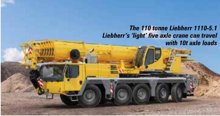
*The 110 tonne Liebherr 1110-5.1 Liebherr's 'light' five axle crane can travel with 10t axle loads*
