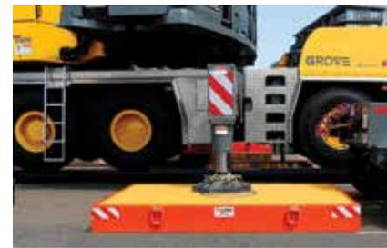
average ground bearing pressure to 5,625psf/26.9 tonnes per square metre which is the objective.
