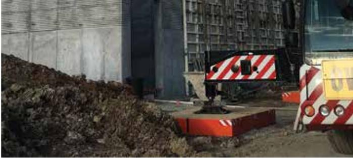
a 50 to 150mm - two to six inch - thick layer of sand may be needed. A downside with using sand is that it is messy.
