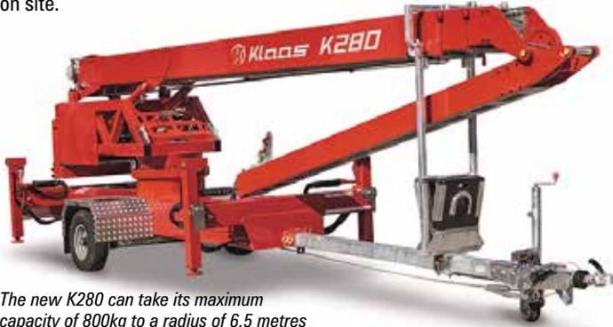
The new K280 can take its maximum capacity of 800kg to a radius of 6.5 metres
