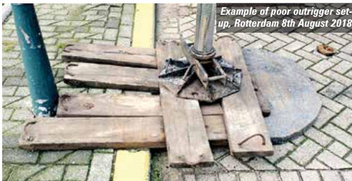
Example of poor outrigger set-up, Rotterdam 8th August 2018
