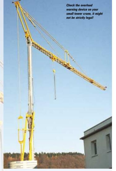
a different light and warning signal must sound continuouly and the controls must lock out.
