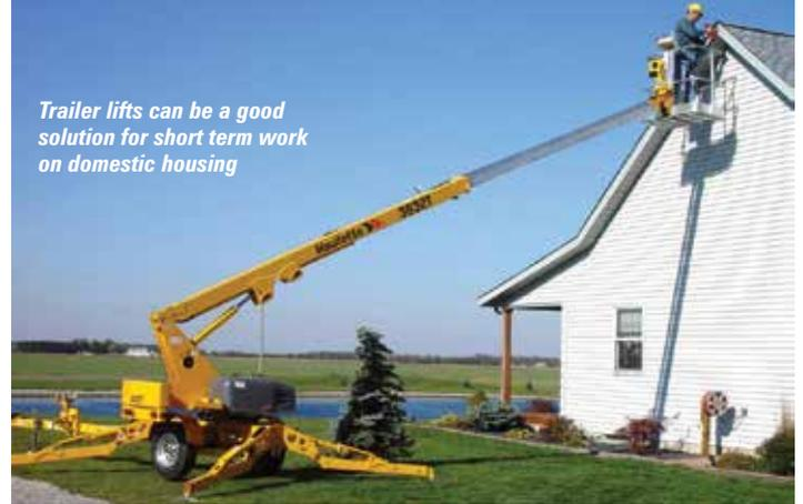
Trailer lifts can be a good solution for short term work on domestic housing
