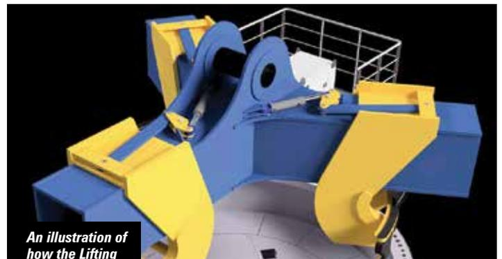
*An illustration of how the Lifting Tool works*
