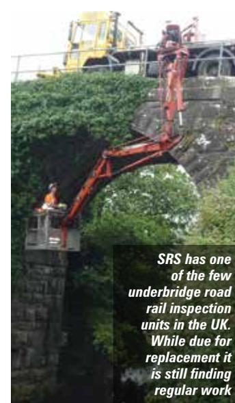
SRS has one of the few underbridge road rail inspection units in the UK. While due for replacement it is still finding regular work
