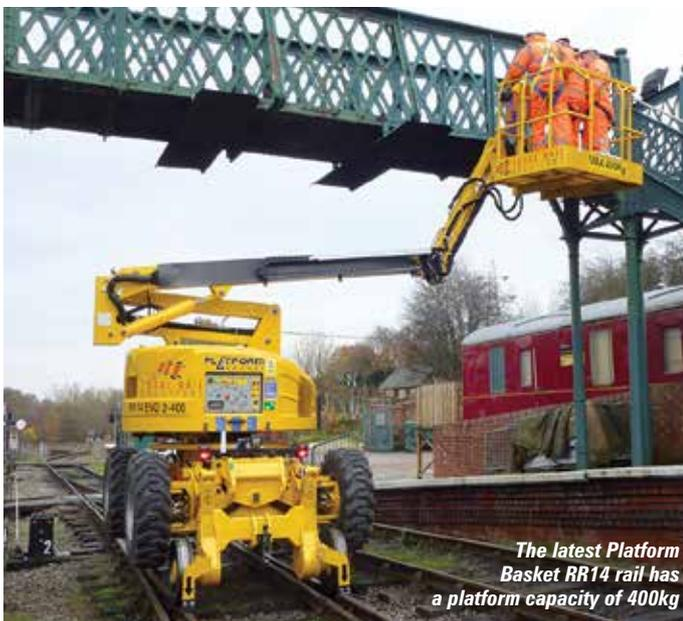
The latest Platform Basket RR14 rail has a platform capacity of 400kg
