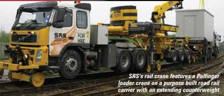
SRS's rail crane features a Palfinger loader crane on a purpose built road rail carrier with an extending counterweight
