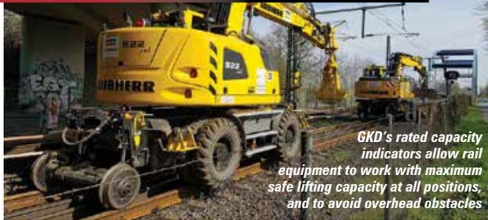
*GKD's rated capacity indicators allow rail equipment to work with maximum safe lifting capacity at all positions, and to avoid overhead obstacles*
