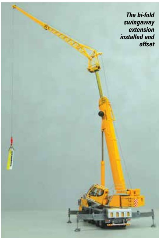
*The bi-fold swingaway extension installed and offset*
