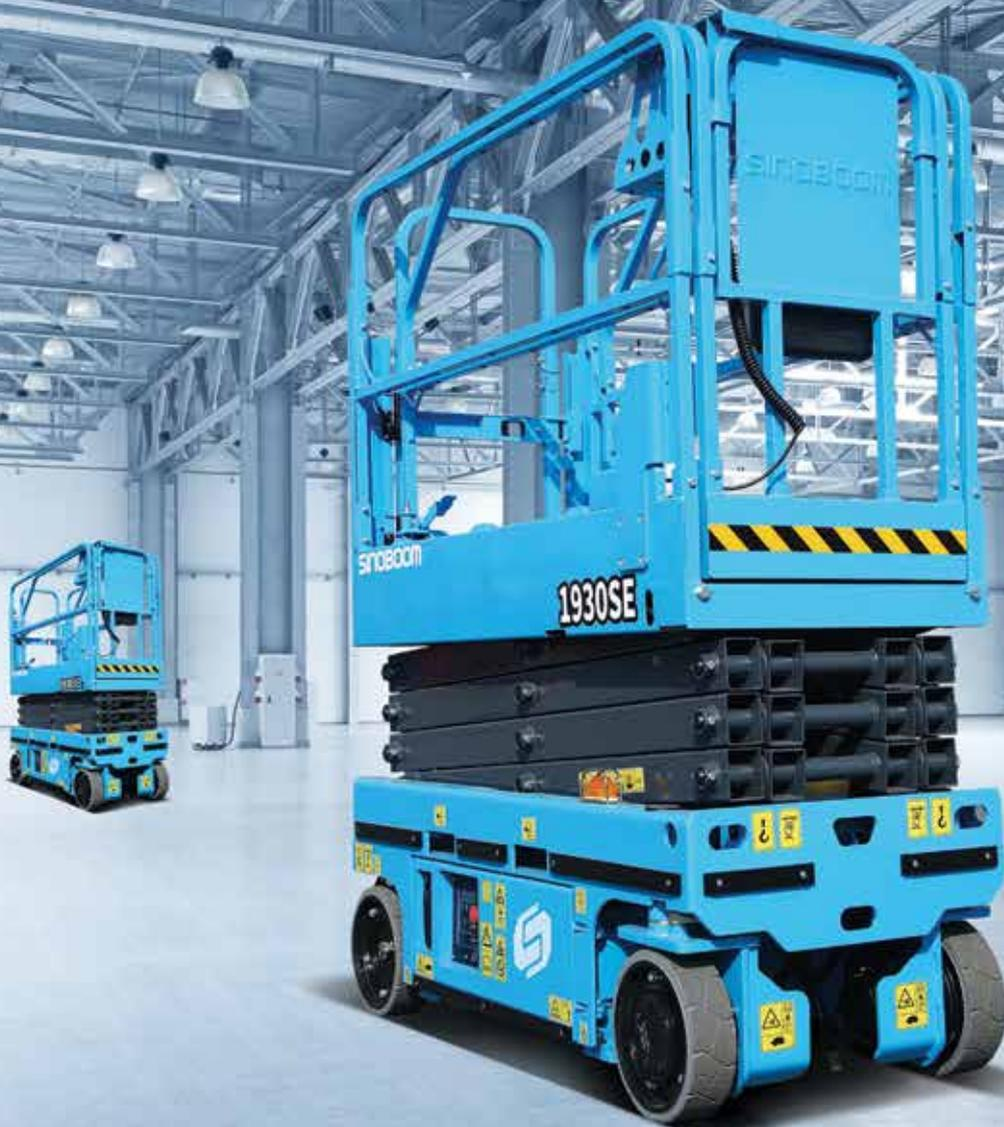
Efficient and environmentally friendly, the Sinoboom electric scissor lift series features platform heights from 4m (12'6") to 14m (45' 3") and offers numerous benefits: exclusive open chassis design for reduced daily maintenance time; bumper rail protection; lower cost of ownership and highly versatile parts and components.
