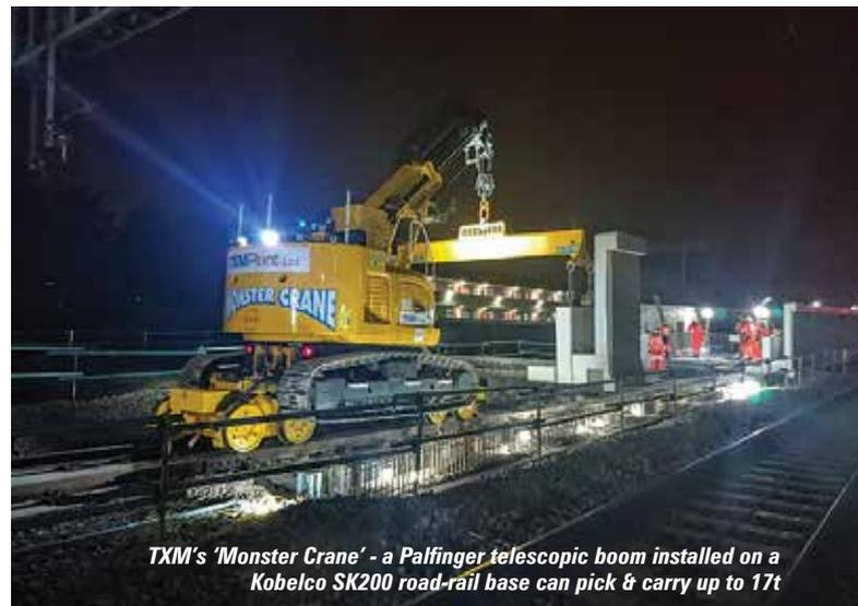
TXM's 'Monster Crane' - a Palfinger telescopic boom installed on a Kobelco SK200 road-rail base can pick & carry up to 17t
