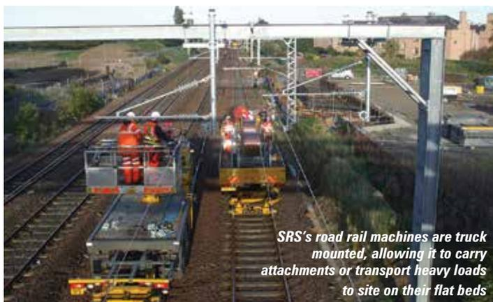
SRS's road rail machines are truck mounted, allowing it to carry attachments or transport heavy loads to site on their flat beds
