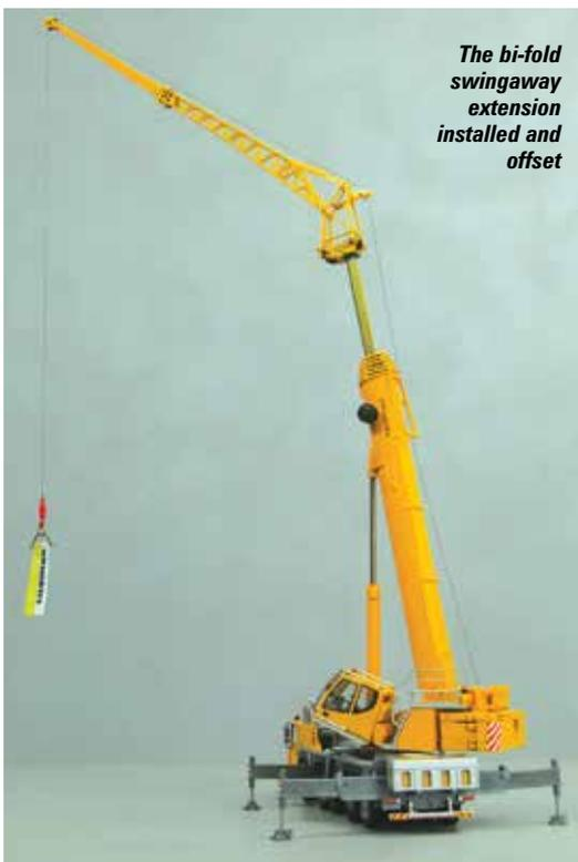
*The bi-fold swingaway extension installed and offset*
