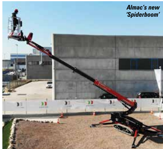
The Spiderboom can drive at heights of up to nine metres
