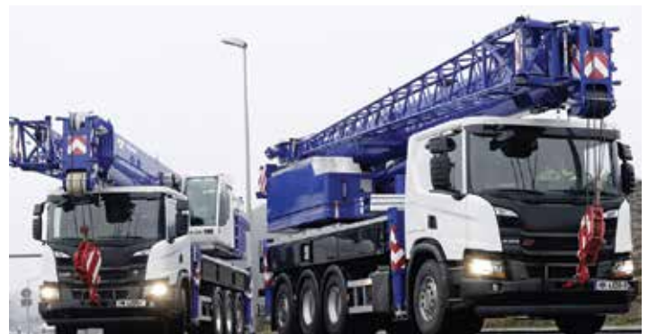
The HK 4.050 and HK 4.070 can travel in working configuration with GVW as low as 32 tonnes
