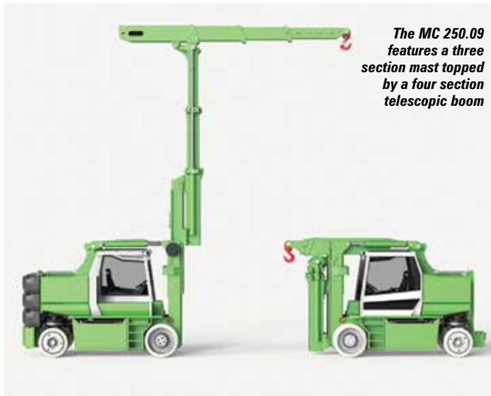
JMG's all new 25 tonne MC 250.09 FL pick & carry forklift type crane
