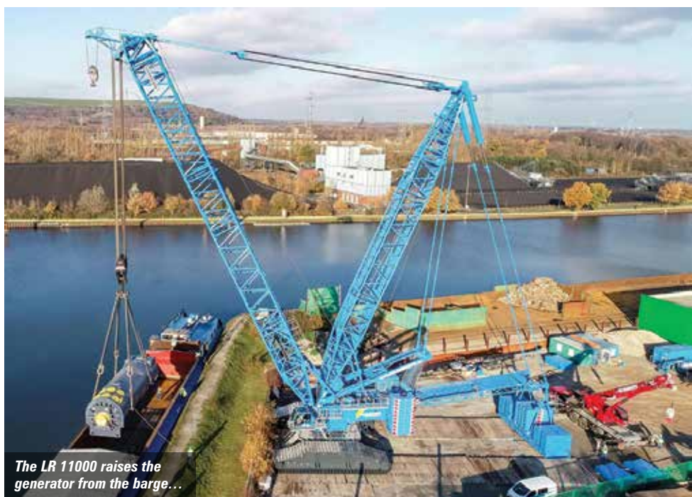
...and tracks in reverse to create space for the SPMTs to drive in below the load
