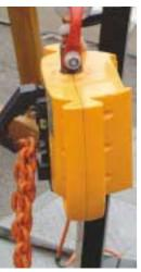
A load is connected to the unit via a chain link or a ring hook, both of which can be applied with one hand, once the load is in position and the unit is relieved of any load a press on the remote control button will drop one end of the chain allowing
