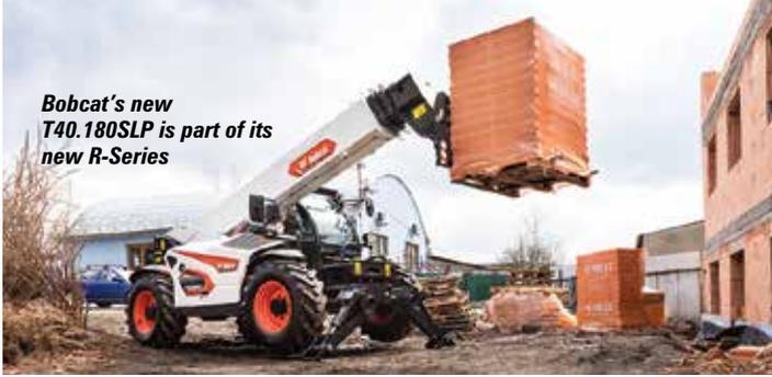
hydrostatic telehandlers with maximum lift heights of seven and nine metres respectively. Both are compact machines powered by a Kubota Stage V engine and with a width and height of no more than two metres.
