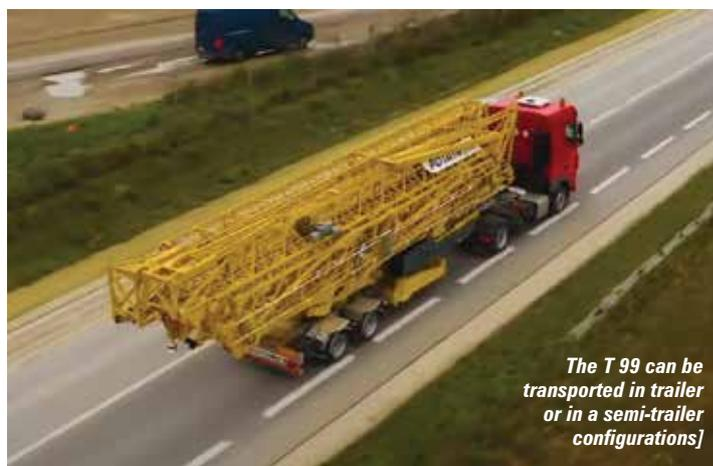
*The T 99 can be transported in trailer or in a semi-trailer configurations]*
