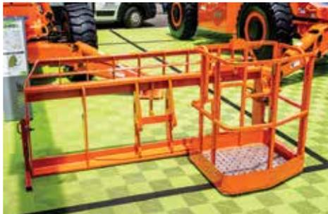
The new Operator Station is attached directly to the fork carriage allowing the operator to ride with the load
