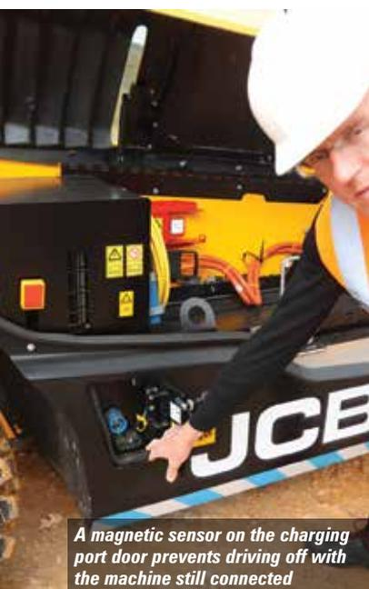
A magnetic sensor on the charging port door prevents driving off with the machine still connected
