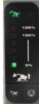
The visual display of JCB's Adaptive Load Control system
