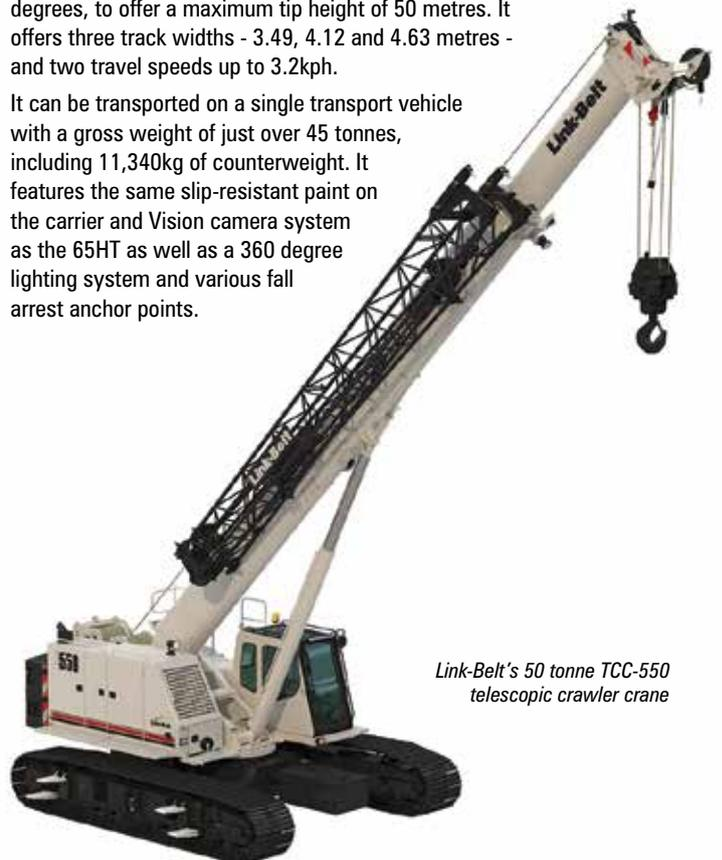
Link-Belt's 50 tonne TCC-550 telescopic crawler crane
