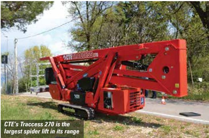
CTE's Traccess 270 is the largest spider lift in its range
