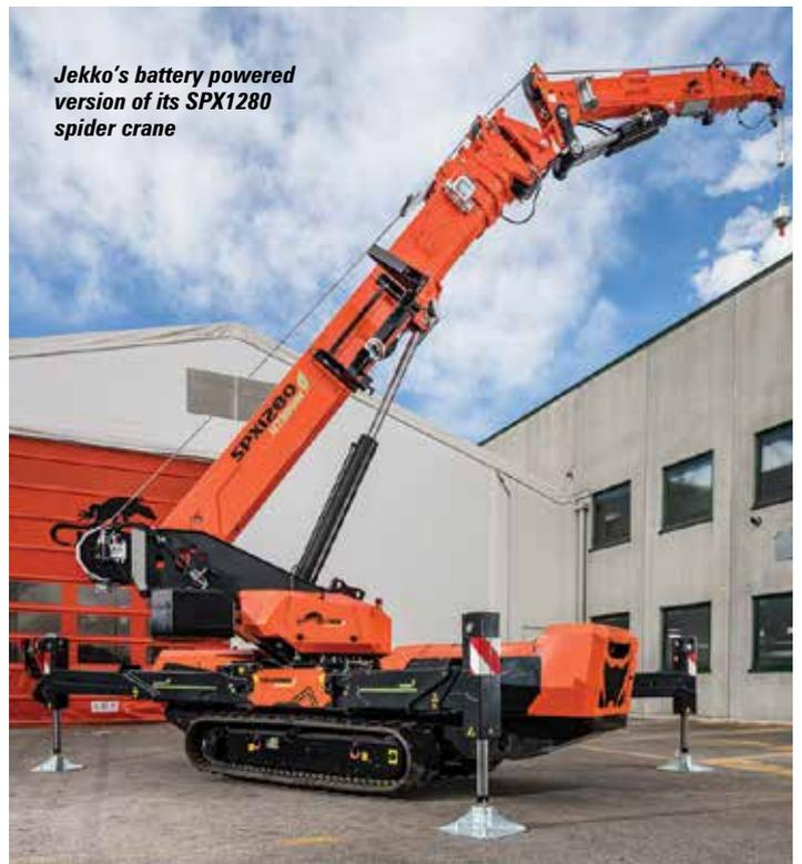
Jekko's battery powered version of its SPX1280 spider crane
