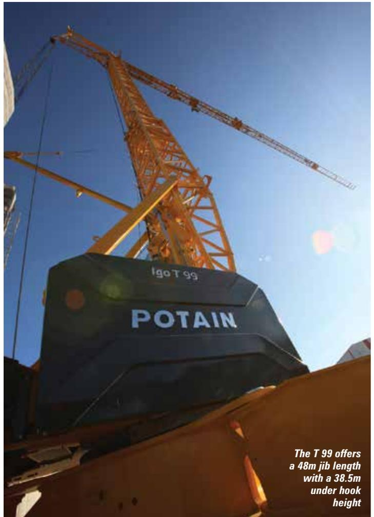
*The T 99 offers a 48m jib length with a 38.5m under hook height*
