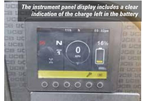
The instrument panel display includes a clear indication of the charge left in the battery
