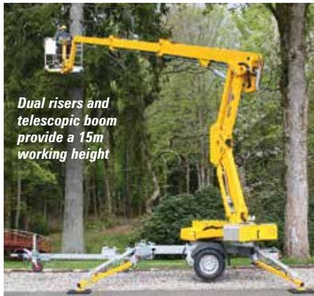
Dual risers and telescopic boom provide a 15m working height
