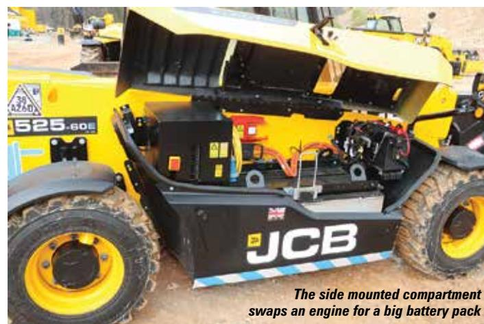
*The side mounted compartment swaps an engine for a big battery pack*
