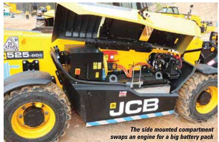
*The side mounted compartment swaps an engine for a big battery pack*
