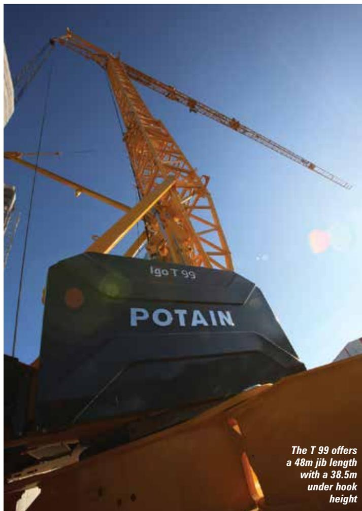
*The T 99 offers a 48m jib length with a 38.5m under hook height*
