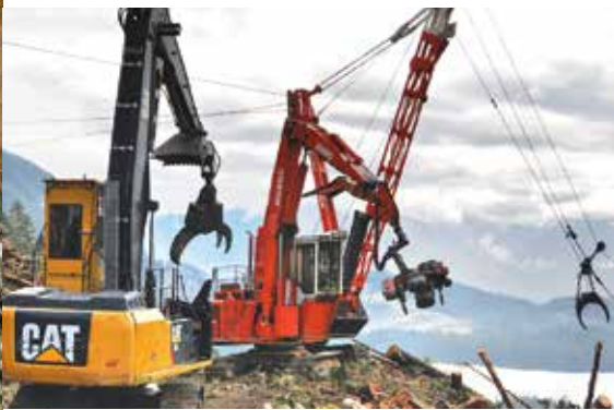
A Madill swing yarder/cable yarder in action brings logs to the nearest road with blocks, grabs and cables
