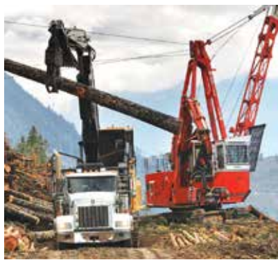
A Madill swing yarder/cable yarder in action brings logs to the nearest road with blocks, grabs and cables
