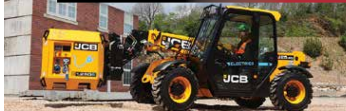
Fork pockets allow the 1.25QE power pack to be easily moved around on site
