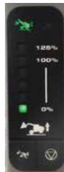
The visual display of JCB's Adaptive Load Control system
