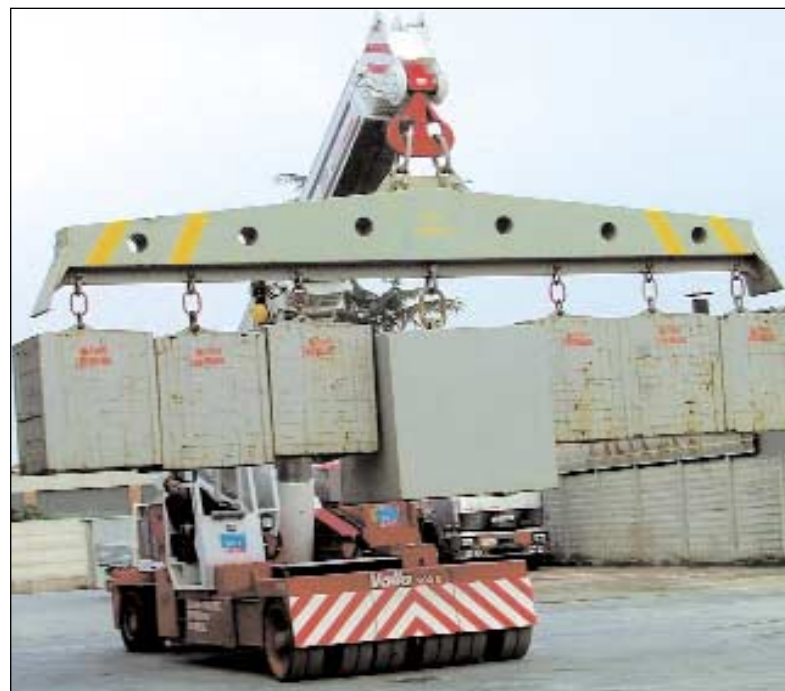
Valla Cranes currently offers the widest range of pick-and-carry cranes in the UK, running from units hardly larger than a pallet truck, to a massive 90-tonne pick-and-carry electric-powered machine (pictured).
