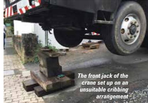
The front jack of the crane set up on an unsuitable cribbing arrangement
