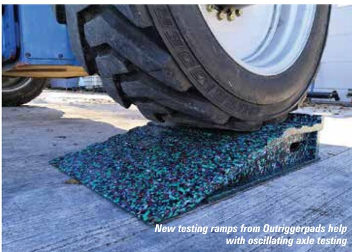
New testing ramps from Outriggerpads help with oscillating axle testing
