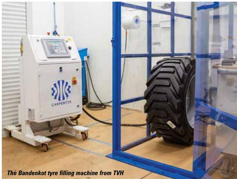
The Bandenkot tyre filling machine from TVH
