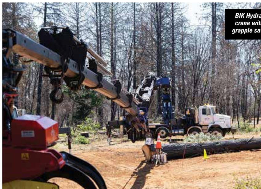
BIK Hydraulics' PM crane with Mecanil grapple saw in action
