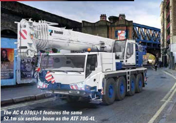
The AC 4.070(L)-1 features the same 52.1m six section boom as the ATF 70G-4L
