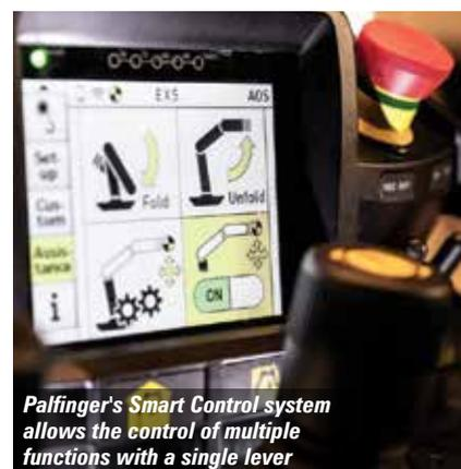
*Palfinger's Smart Control system allows the control of multiple functions with a single lever*
