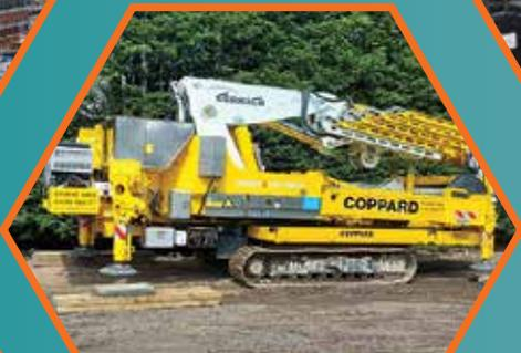
Coppard's 30 tonne Cormach 240000AX loader crane on tracks
