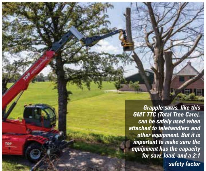
Grapple saws, like this GMT TTC (Total Tree Care), can be safely used when attached to telehandlers and other equipment. But it is important to make sure the equipment has the capacity for saw, load, and a 2:1 safety factor
