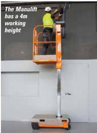
The Manulift has a 4m working height
