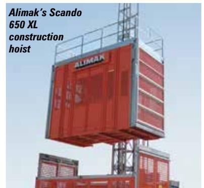
Alimak's Scando 650 XL construction hoist
