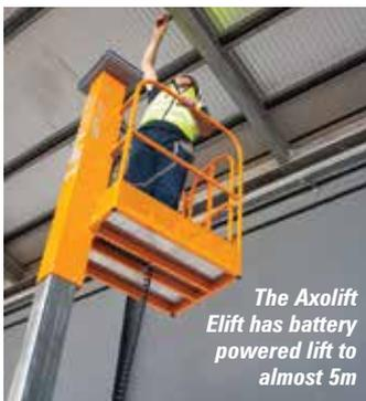
The Axolift Elift has battery powered lift to almost 5m
