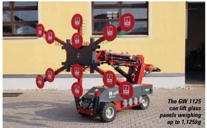
The GW 1125 can lift glass panels weighing up to 1,125kg
