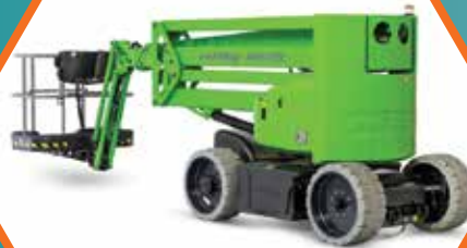
Niftylift's HR17NE 50ft all electric boom lift
