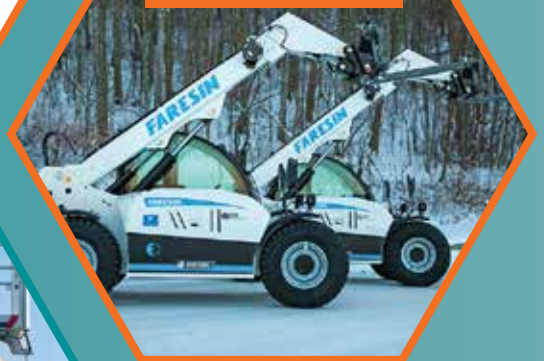
The Faresin 6m/2,600kg Faresin 6.26 full electric telehandler
