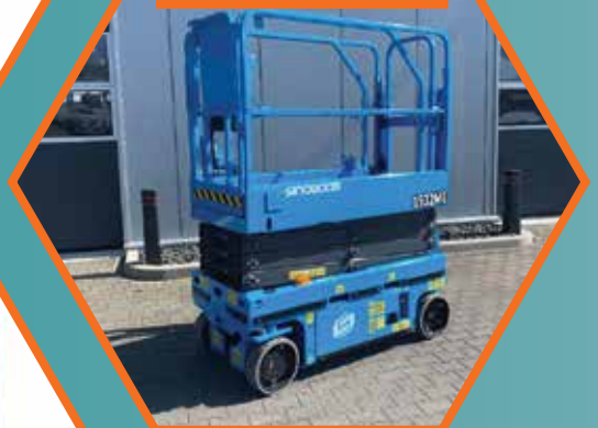
Sinoboom's 19ft 1932ME slab electric scissor lift
