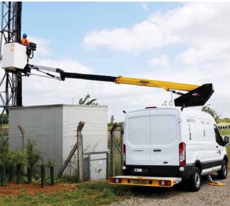
Versalift's type approved VTL-136 is available on a Ford Transit chassis
