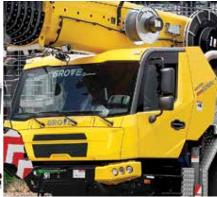
The latest Grove cranes, such as the new long boom GMK3060L-1 feature new carrier cabs, which meet the latest crash test requirements, and offer operators improved visibility and comfort
