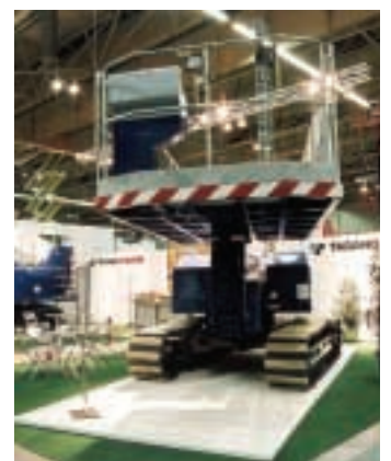
Tadano's Super Deck - a scissor lift sized platform on a stick! It offers a lift capacity of up to 800 kilograms and up to eight metres of outreach.
