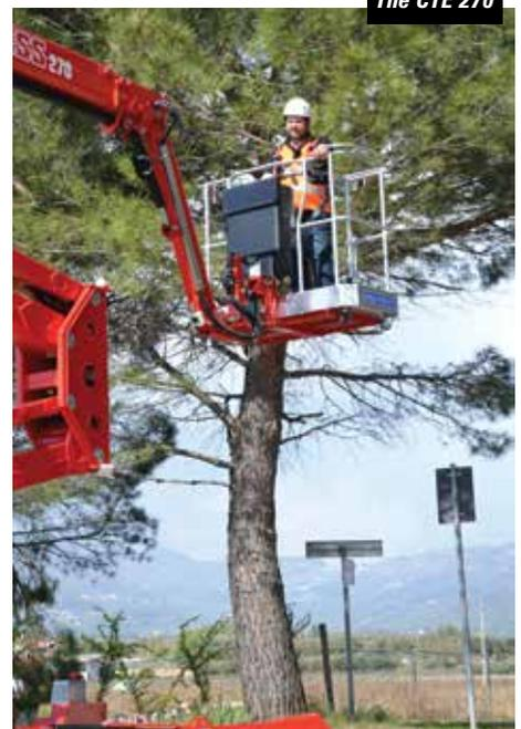
power is Kubota diesel, which is available with an additional AGM battery pack, good for around an hour's continuous operation. It can also be operated while plugged in and recharging, so in essence three power sources on the same machine.
