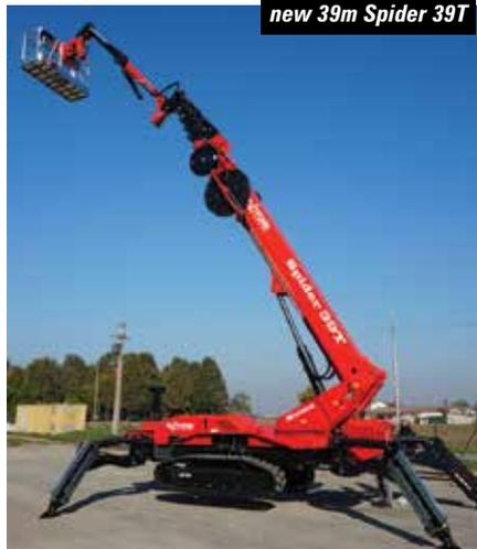
and it can be ordered as a diesel/lithium-ion hybrid or with diesel/AC electric power. It joins the company's 30 metre Spider 30 T and its 43 metre 43 T.
