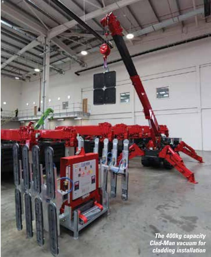
The 400kg capacity Clad-Man vacuum for cladding installation
