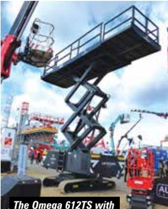
**The Omega 612TS with rotating scissor stack**
