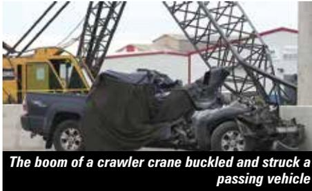
The boom of a crawler crane buckled and struck a passing vehicle
