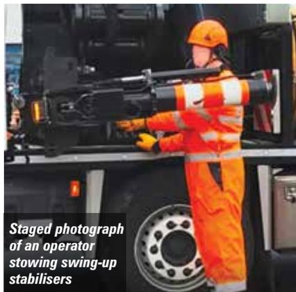
Staged photograph of an operator stowing swing-up stabilisers
