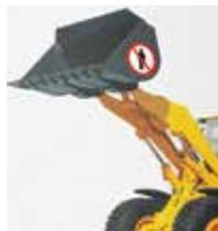
Brothers Steel and Quinlen Adams had been lifted in the loader's bucket to a height of around 4.5 metres in order to carry out repairs to the suction lines of a sand washing machine at the company's sand mine in Chevallum, Queensland. The bucket began to tilt forward, causing Quinlen to jump to a steel crossbeam for safety, while Steel suffered serious injuries after striking his head on the bucket.
