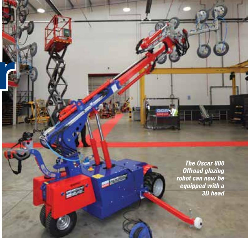
The Oscar 800 Offroad glazing robot can now be equipped with a 3D head
