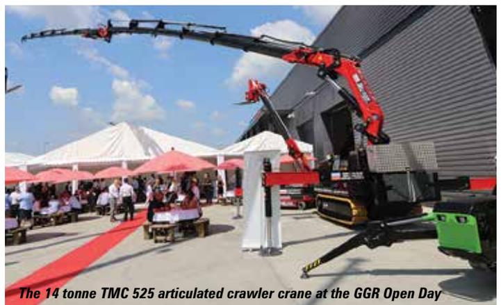
The 14 tonne TMC 525 articulated crawler crane at the GGR Open Day
