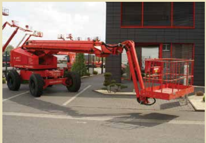
The unique TKD triangular boom profile
