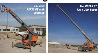
11.5 tonnes on full boom or take 1.3 tonnes out to a radius of 21.5 metres and can pick & carry up to five tonnes. Remote controls and air conditioning are standard, while options include a 13 metre lattice extension which takes the maximum tip height to almost 40 metres with a 1.5 tonne capacity, and a work platform. The crane has an overall length of 5.45 metres an overall width of 2.5 metres and a stowed height of 3.27 metres.
