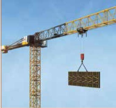
**Liebherr** adds the 10 tonne 205 EC-B 10 flat top tower crane with the first units sold in France and Italy.
