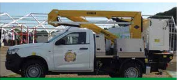
**Versalift** unveils its new 13.5 metre VTA135-H pick-up mounted platform with a 500kg cargo payload.
