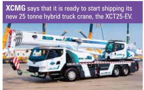
**XCMG** says that it is ready to start shipping its new 25 tonne hybrid truck crane, the XCT25-EV.
