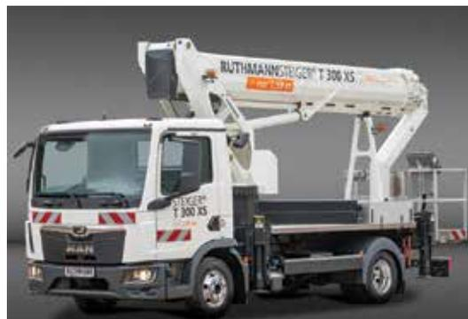
**Ruthmann** unveils a redesigned compact version of its 30 metre T 300 truck mount - the T 300 XS (Xtra Short).
