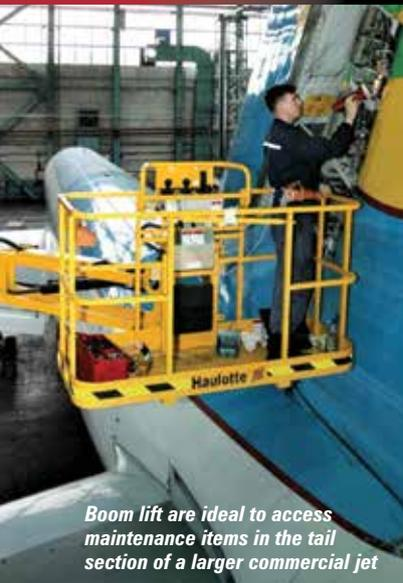
Boom lift are ideal to access maintenance items in the tail section of a larger commercial jet
