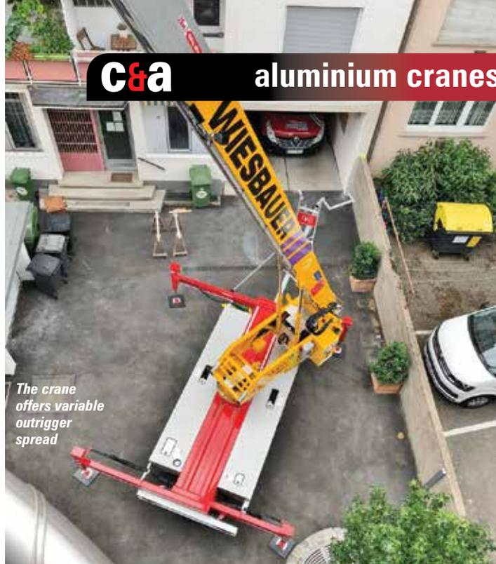
*The crane offers variable outrigger spread*
