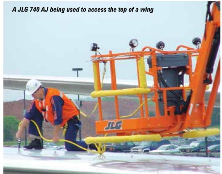
A JLG 740 AJ being used to access the top of a wing
