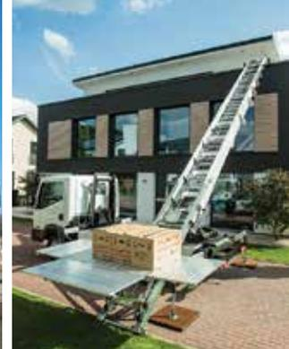
Böcker's smallest model, the Top Lift, takes this approach. It comes in three versions (Basic, Standard, and High Speed) able to reach heights of 20.3 metres, differentiated by capacity - the Basic lifts 150kg, the Standard 250kg and the High Speed 230kg - and, as the name of the last version suggests, hoisting speed. Böcker now offers a specialised platform for lifting solar panels.
