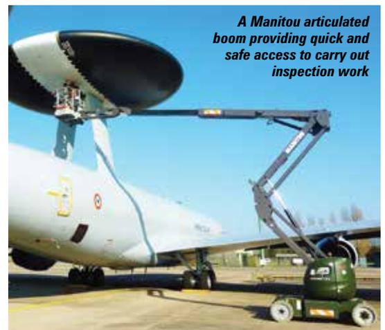
**A Manitou articulated boom providing quick and safe access to carry out inspection work**
