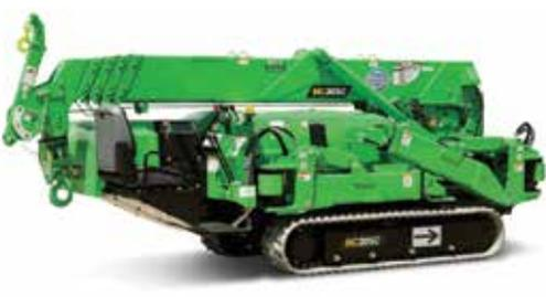
**Kranlyft** launches the new 2.98 tonne Maeda MC305CB-3 electric powered spider crane.
