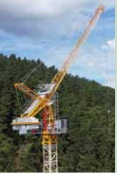
**Jaso** announces an 18 tonne J198HPA hydraulic luffing tower crane with the first five units going to UK rental company **Falcon Tower Crane Services**.
