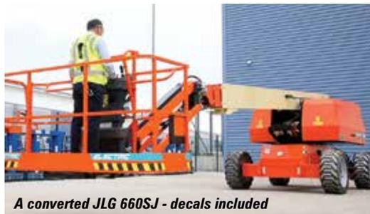
The pack is aimed at extending the working life of existing boom lifts as demand for emission free models increases. Covered by the JLG warranty programme, lead acid conversion kits are available now with the lithium version due in the spring.
