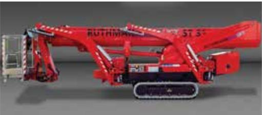
**Ruthmann** unveils the **Bluelift** ST31 telescopic spider lift using the new five section boom and articulated jib from the Ruthmann T 330 XS truck mount.
