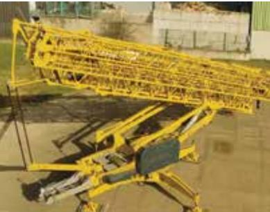
**Potain** unveils the six tonne Igo T 99 self-erecting tower crane with 48 metre jib and 38.5 metre under hook height.
