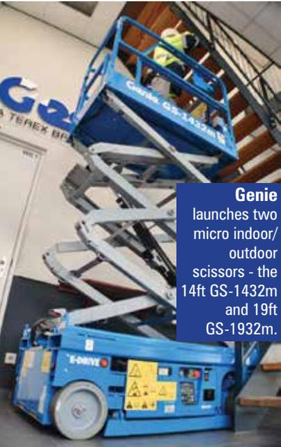
**Genie** launches two micro indoor/outdoor scissors - the 14ft GS-1432m and 19ft GS-1932m.
