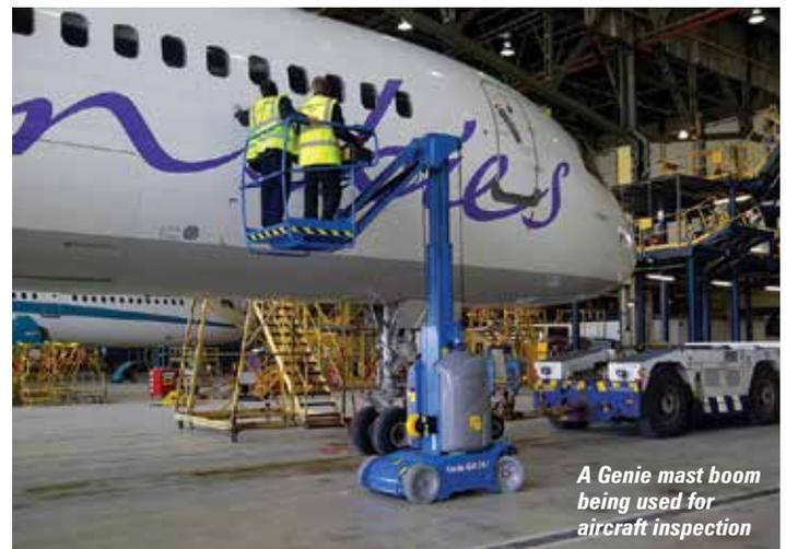
A Genie mast boom being used for aircraft inspection
