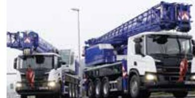
**Tadano** launches the 50 tonne HK 4.050-1 and 70 tonne HK 4.070-1 truck mounted cranes on commercial chassis.
