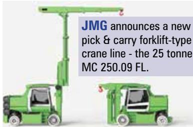
**JMG** announces a new pick & carry forklift-type crane line - the 25 tonne MC 250.09 FL.
