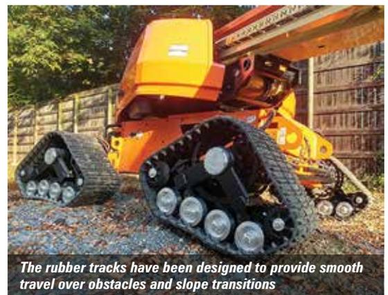
The rubber tracks have been designed to provide smooth travel over obstacles and slope transitions
