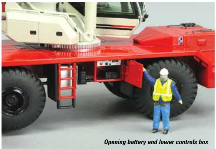
*Opening battery and lower controls box*
