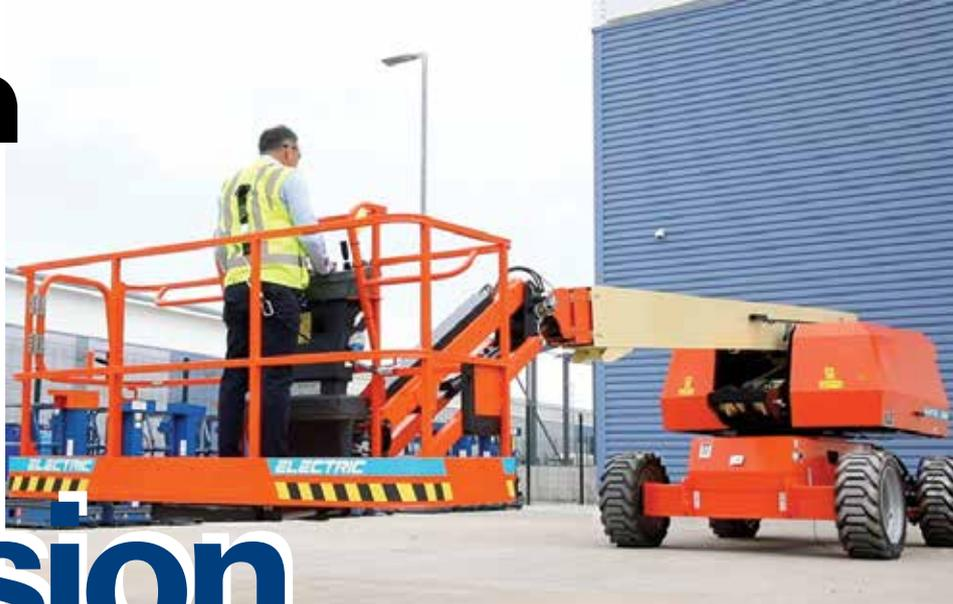
With the growing demand for low or zero emission equipment, a question that comes to mind concerns the impact on the economic life of existing diesel powered machines, especially the larger more expensive models. JLG has developed a possible solution in the form of a retrofit kit to convert diesel powered boom lifts - starting with the 66ft 660SJ telescopic - to battery electric power.
