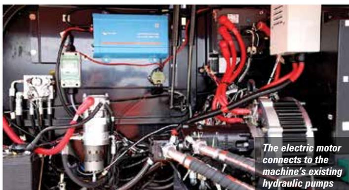
The electric motor connects to the machine's existing hydraulic pumps
