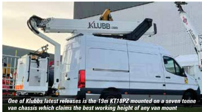
One of Klubb's latest releases is the 19m KT18PZ mounted on a seven tonne van chassis which claims the best working height of any van mount
