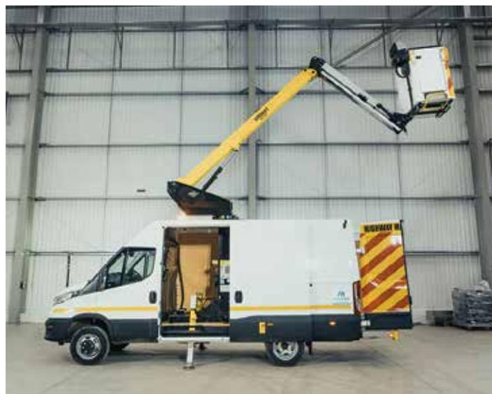
in the region of 17 metres. Although the larger vans need additional driving licence requirements for younger operators, their main advantage is the much larger cargo carrying capacity - up to 2,300kg when mounted on the largest chassis.
