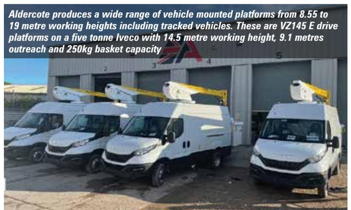
Aldercote produces a wide range of vehicle mounted platforms from 8.55 to 19 metre working heights including tracked vehicles. These are VZ145 E drive platforms on a five tonne Iveco with 14.5 metre working height, 9.1 metres outreach and 250kg basket capacity
