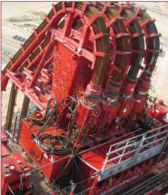
If you are not familiar with them, strand jacks use hydraulic jacks and rope clamps to pull or let out multiple strands of wire rope. A strand jack - in most operations - remains stationary relative to the load and pulls the rope through itself, moving the load attached to the ropes. Multiple strand jacks can be used together, to lift hundreds or thousands of tonnes. Strand jacks can be positioned using nothing more than a pick & carry industrial crane.
