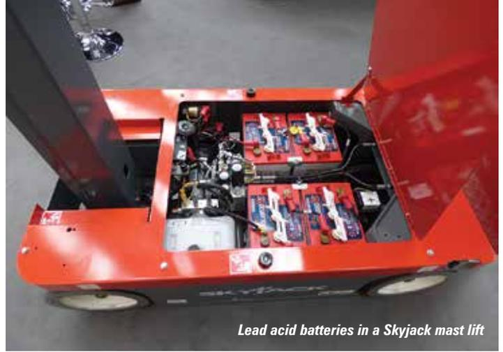
Lead acid batteries in a Skyjack mast lift
