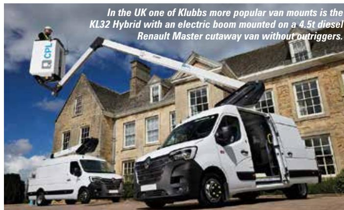
In the UK one of Klubb's more popular van mounts is the KL32 Hybrid with an electric boom mounted on a 4.5t diesel Renault Master cutaway van without outriggers.
