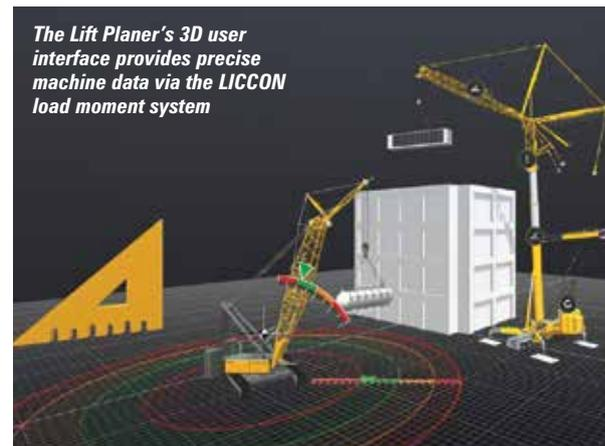
The Lift Planner's 3D user interface provides precise machine data via the LICCON load moment system
