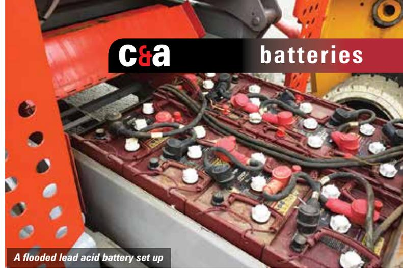
A flooded lead acid battery set up
