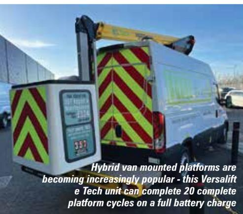
Hybrid van mounted platforms are becoming increasingly popular - this Versalift e Tech unit can complete 20 complete platform cycles on a full battery charge
