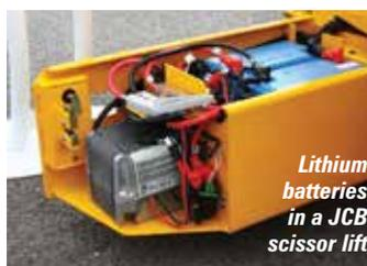
Lithium batteries in a JCB scissor lift
