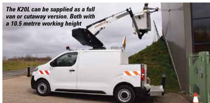
The K20L can be supplied as a full van or cutaway version. Both with a 10.5 metre working height
