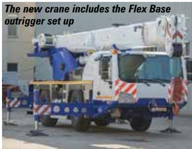
The new crane includes the Flex Base outrigger set up
