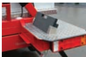
Neat outrigger pad provision and storage on a Ruthmann truck-mounted boom lift.
