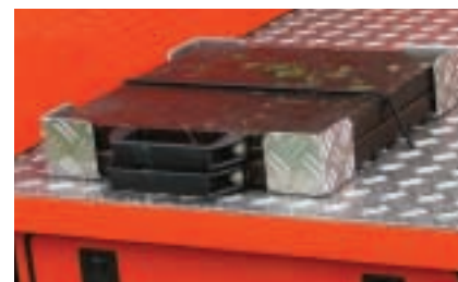
Outrigger pad provision and stowage on a Bison 3.5-tonne truck-mounted platform, now part of the Palfinger portfolio.
