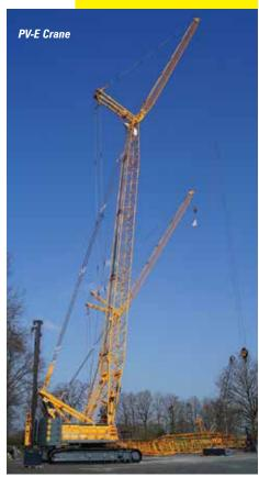
zero emission cranes can run for a full eight hour shift before requiring a re-charge. Batteries are removable and can be re-charged off site if on site charging facilities are not available. The company will offer both lattice and telescopic boomed models from 80 to160 tonnes capacity for the lattice and 70-120 tonnes for the telescopics.
