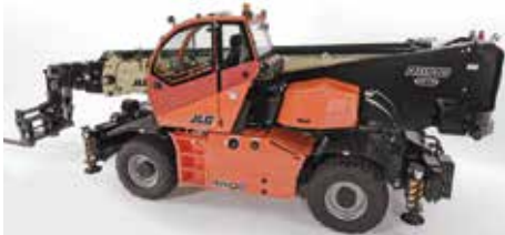
The 30 metre/5,000kg R11100 - JLG machines are based on Dieci's latest Pegasus models
