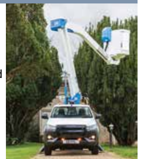
CPL's 4x4 Isuzu D-Max pick-up mounted platform
