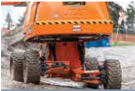
JLG's '670SJ Self-Leveling' boom has a working height is 22.3 metres with a maximum outreach of 17.5 metres
