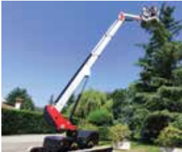
The U-1570 Evo uses Multitel's aluminium boom coupled with AlmaCrawler's bi-levelling tracked undercarriage
