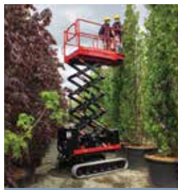
The Bibbi 870-BL Evo has an 7.9 metre working height and 250kg capacity
