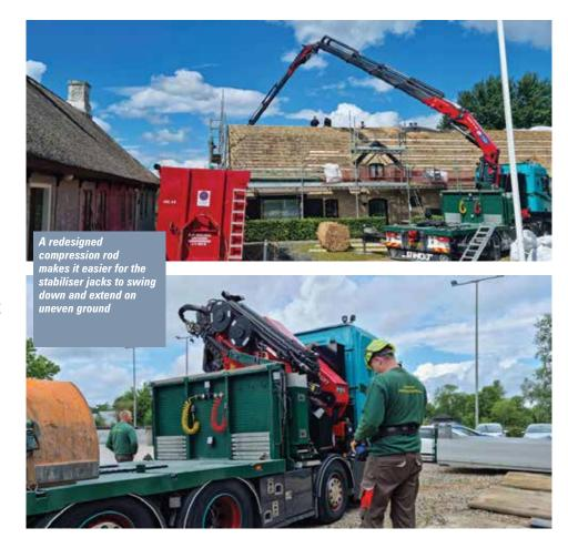
shortened, but if it is not loosened again before stowing, the entire rod could be damaged. Much of Svenstrup's work takes place on uneven construction sites, with many obstacles to clear when extending the outrigger beams.
