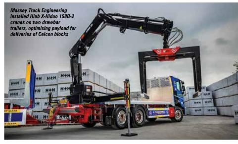
"These vehicles are truly one of a kind, with a 28t payload using a 26t drawbar combination. There is nothing quite like them currently in the UK. The weight reduction gives a significant additional
