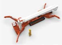
"The new RA53 will be equipped with an undercarriage that can be extended both vertically and horizontally with a dynamic self-levelling system, developed to compensate for slopes," adds Vender. "It's separately extendable tracks will guarantee greater stability on rough and steep terrain and, in wide position, the height from the ground will increase to improve stability on uneven surfaces."
