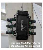
Lightning Protection Systems check, with the technician controlling it from the nacelle.
