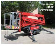
The new model is similar in concept to Hinowa's 33 metre model which has a four section lower boom/riser and three section upper boom, with the 40 metre unit having longer boom sections. The maximum capacity is 300kg through most of the working envelope, reducing to 230kg for the last metre of outreach or when the upper boom is fully elevated when the lower boom remains stowed.
