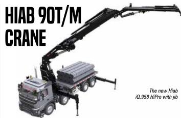
Hiab is to launch a new 90 tonne/metre loader crane - the iQ.958 HiPro - its second model in its new iQ range. The iQ.958 HiPro's nine section boom and seven section jib use the new 12 sided, V12 profile resulting in a light compact crane with a minimum width of just under two metres, allowing it to be installed on smaller trucks within the four axle 32 tonnes GVW category.
