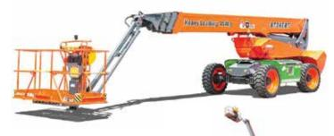
all electric BT34ERT and diesel BT34RT with four section booms and articulated jibs for a maximum working height of 34.1 metres and a maximum platform capacity of 454kg.
