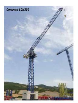
60 metres to offer a jib tip capacity of up to 3.4 tonnes. The crane has a minimum working radius of four metres and a minimum out of service radius of nine metres.
