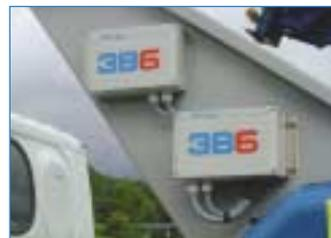
The duplicate systems of the 3B6 system for full redundancy.
