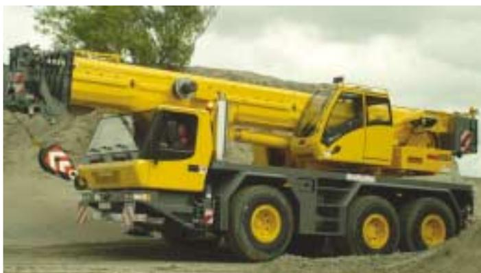
Runcorn-based Quigley Crane Hire recently looked to its 350 tonne capacity Demag AC350 SS2 mobile crane to lift a 3 tonne bronze sculpture onto the new Peel Holdings building at Trafford Quays, Manchester. A 46.9-metre main boom combined with a 48-metre luffing jib provided the necessary up-and-over reach for the delicate lift to height of 42 metres and a radius of 56
