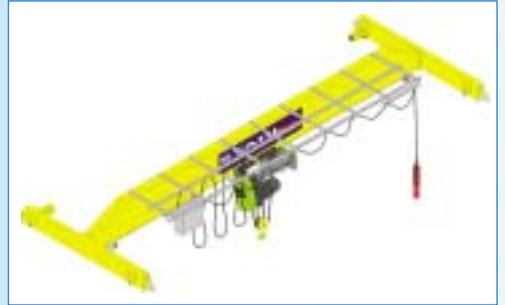
R Stahl says that a 25-tonne capacity double-girder kit will be available later in the year with a varying span from 6 to 22 metres, lift heights ranging from 6- to 10 metres and hoist speeds from 3.2/0.5 to 7.5/1.5 metres per minute. All kits use standard calculations, connections, easy to obtain materials, continuous load monitoring technology and various other safety features.
