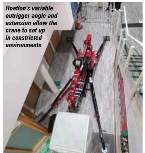
Luffing jibs, like that on this Hoeflon, allow spider cranes to reach under roofs
