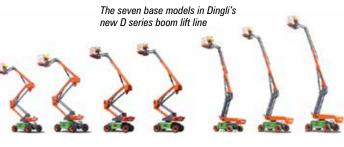
range comprises seven base models including four articulated boom lifts - 46ft, 53ft, 59ft and 66ft with working heights 16, 18, 20 and 22 metres - plus three telescopics - 46ft, 53ft and 59ft with working heights of 16, 18 and 20 metres. All seven are available with three power options all-electric, hybrid or diesel making 21 different variants.
