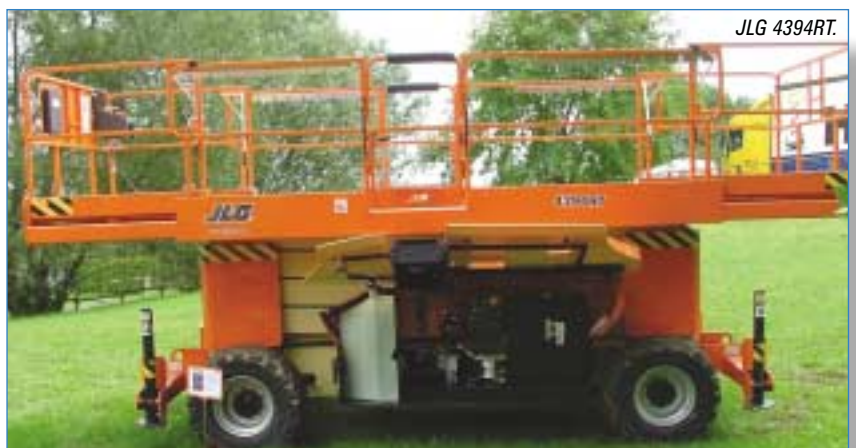
Fig 3. RT scissors with lift capacity of 900 kg plus
