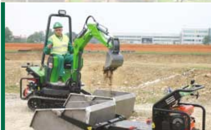
Merlo's Cingo range of small hydrostatic tracked carriers includes a 400-, 600-, 800- and 1000-kilogram capacity version that may in the future be developed into a dedicated access platform or mini crane.
