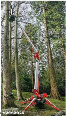
aluminium boom topped by a jib with 180 degrees of articulation. Finally, the 25 metre SMX 250.2 spider lift with variable position outrigger set up will round out the display.
