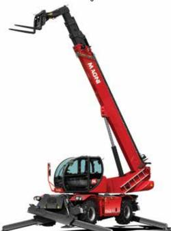
360 degree telehandlers with lift heights up to 51 metres and capacities up to 50 tonnes. For industrial applications the company now offers a specific product range with capacities from 4.5 to six tonnes. On the stand will be the six tonne/30 metre RTH 6.30 360 degree telehandler as well as a selection of attachments.
