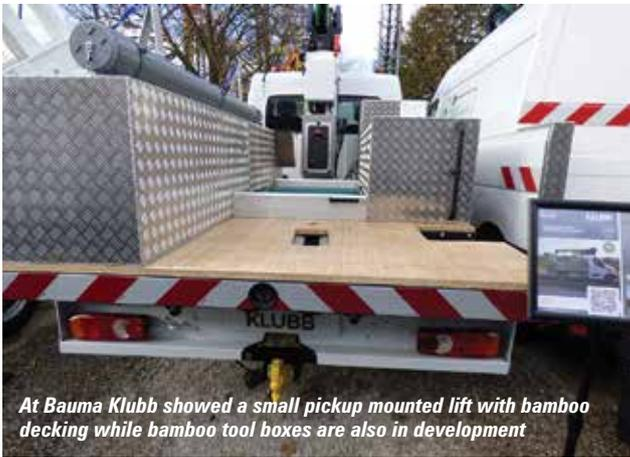
At Bauma Klubb showed a small pickup mounted lift with bamboo decking while bamboo tool boxes are also in development
