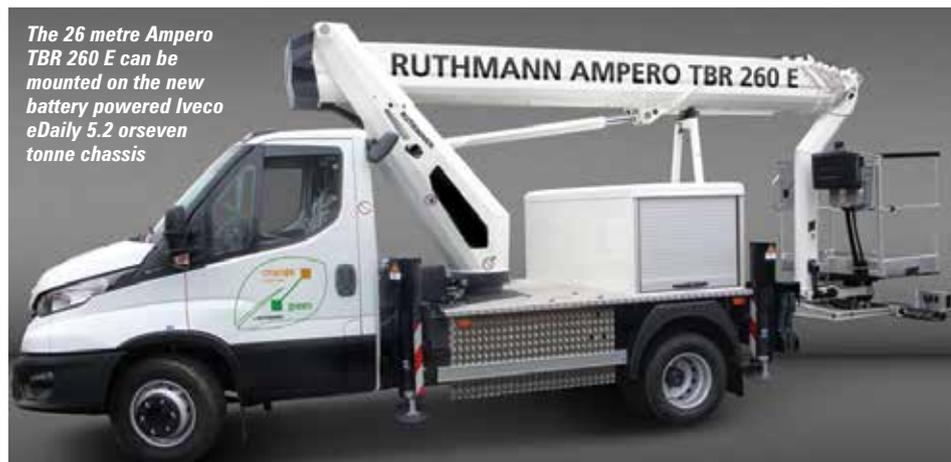
*The 26 metre Ampero TBR 260 E can be mounted on the new battery powered Iveco eDaily 5.2 or seven tonne chassis*
