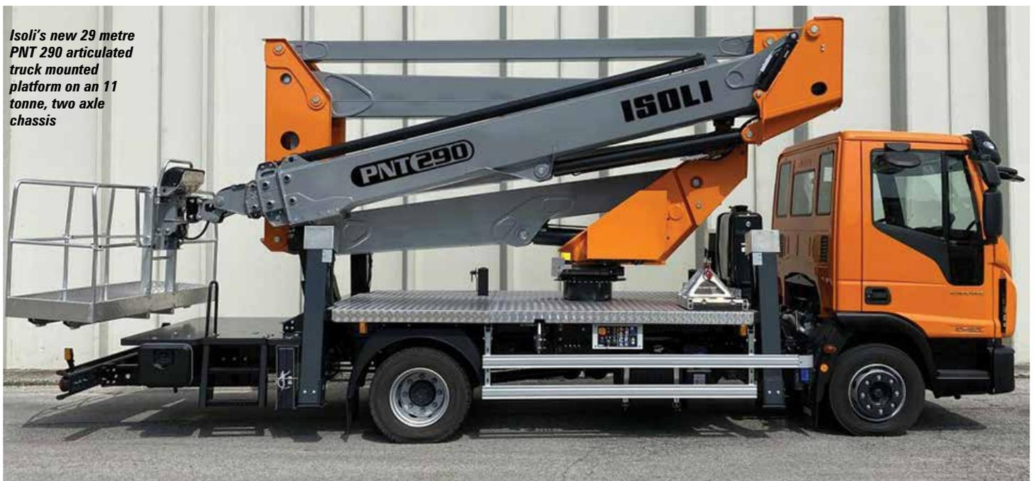
*Isoli's new 29 metre PNT 290 articulated truck mounted platform on an 11 tonne, two axle chassis*
