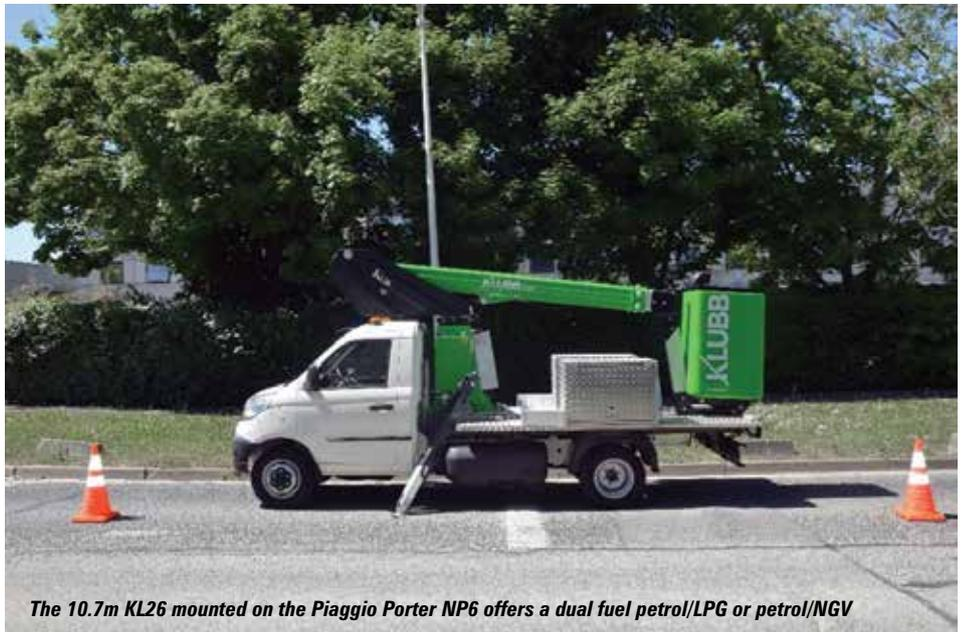
The 10.7m KL26 mounted on the Piaggio Porter NP6 offers a dual fuel petrol/LPG or petrol/NGV
