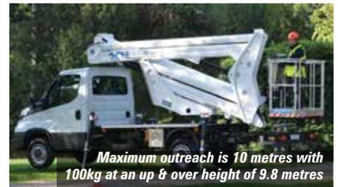
Maximum outreach is 10 metres with 100kg at an up & over height of 9.8 metres
