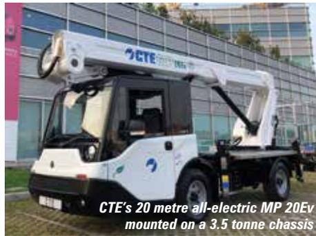
CTE's 20 metre all-electric MP 20Ev mounted on a 3.5 tonne chassis
