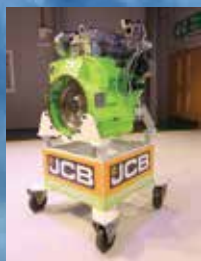
The prototype 532-70 telehandler with (insert) the JCB hydrogen internal combustion engine that powers it
