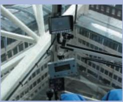
ORLACO Products of The Netherlands has introduced a Compact LCD colour screen for use with cranes. When used with up to three compatible zoom cameras, the screen presents the crane operator with full visibility of the areas surrounding the crane, which would otherwise be impaired, such as the load being lifted and the area around the crane's winch.
