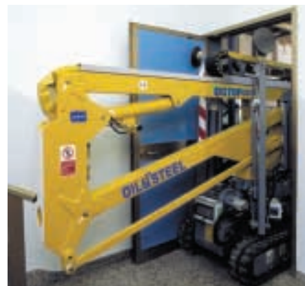
Oil & Steel's Octopussy unit is a hybrid with a trailer chassis from which the machine detaches, allowing it to become a self-propelled unit.
