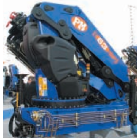
PM's new 60 t/m, nine-extension 63 SP knuckle boom capable of reaching up to 26 m with a four-extension hydraulic jib.
