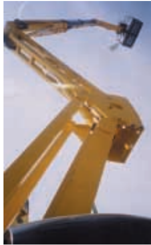
Italian aerial platform producer, Tigieffe, introduced its new 23.1 m working height rough terrain articulating boom, the Airo SG2100-JD4WD. The unit shares the same chassis as its SG21800 predecessor, but includes an additional third boom extension.
