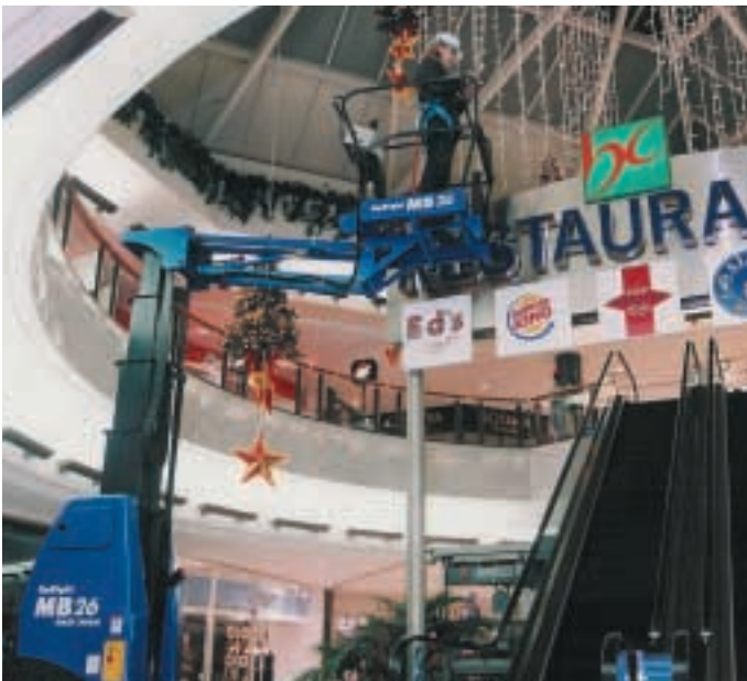
UpRight says that its relatively new powered platform breed, the MB range, which includes the 10 metre working height MB26 (pictured), sits in between a scissor and a boom lift.
