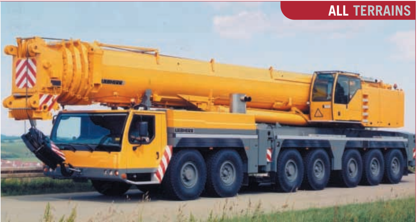
Liebherr states that all of its cranes can be configured to travel with loads of 12.5 tonnes per axle, including this new 400 tonne capacity LTM 1400/1.
