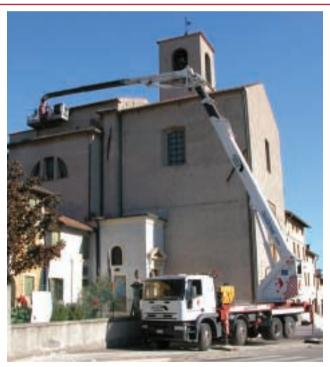
PANTHER PLATFORM Rentals has purchased what will be the UK's first Oil & Steel Eagle 4430 truck mounted platform, to be handed over to the company at Bauma 2004. The 44 metre working height platform provides 30 metres of outreach and features a jib that can be angled up to plus 170 degrees, and also a 360 degree rotating turret.
