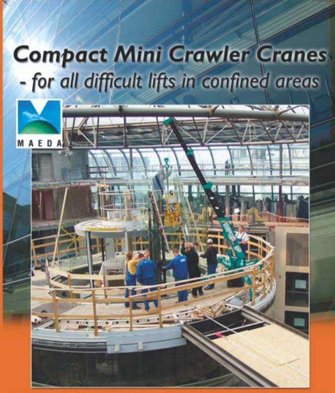
Narrow width (only 600 mm, MC 104) • Long fully automatic pentagonal booms up to 15,6 metres
