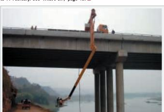
ITALY-BASED PLATFORM producer, Barin SpA, has delivered one if its AB 17 under-bridge inspection units to Sichuan Chengnan of China for inspection and maintenance work on the Chengdu-Nanchong expressway project. The unit, mounted on a Volvo FM12 LHD, 8 x 4 truck chassis, provides a horizontal underbridge reach of 17 metres and a vertical underbridge depth of 21 metres. ■
