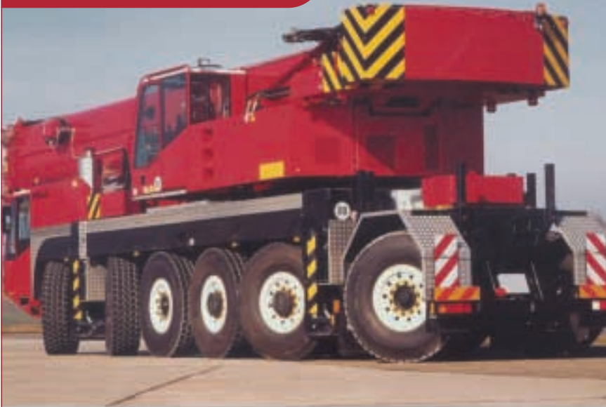
Above: Germany-based crane producer Demag introduced the option of an extra “modular” axle on its mobile cranes, such as this AC 100, to create lower axle weights, and to allow transportation with increased counterweight.
