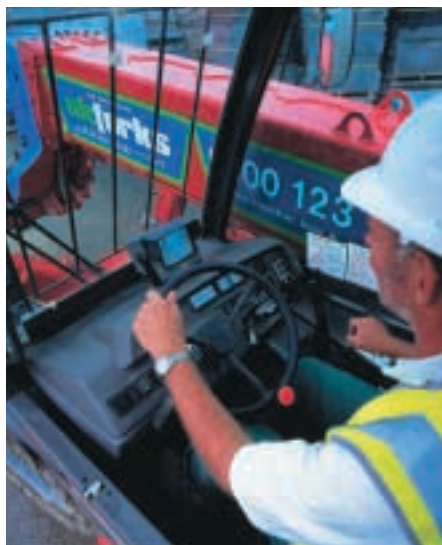
This dash-mounted display monitor of a Manitou MT1233S supplied by UK Forks receives images from a camera on the rear of the vehicle, providing the driver with an easy rear view to eliminate blind spots, while also aiding safe reversing.
