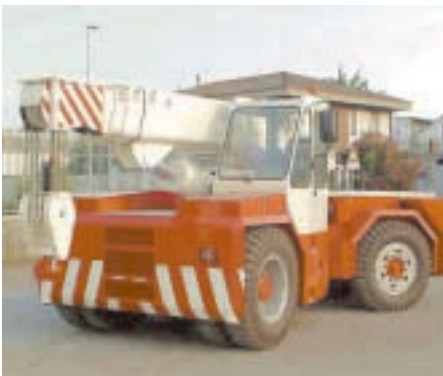
Above: Christiani recently launched its CT300Y with articulated steering, similar to that used on wheeled loaders.
