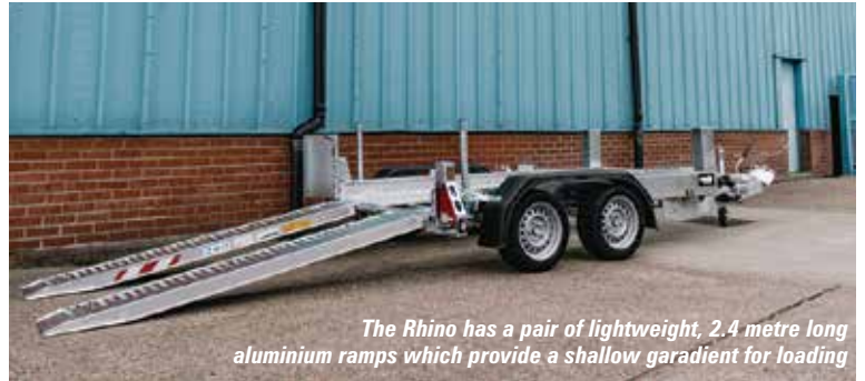
The new two axle Rhino Access Platform Trailer from Towmate Trailers has a 2,995kg payload
