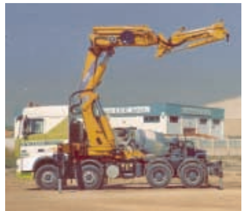
All new large Effer knuckle boom feature continuous slewing, which Effer says is how it defines its large knuckle boom cranes. Pictured here is its 135 tonne/metre 1350 model.
