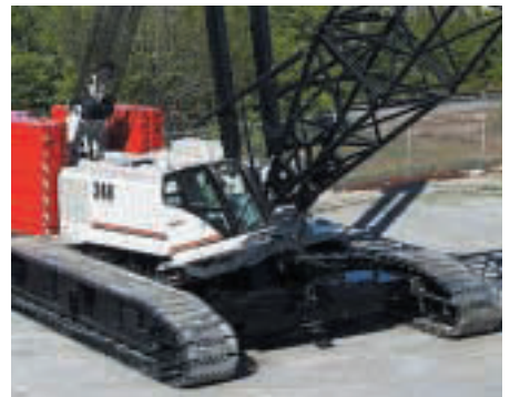
(Above) Link-Belt's new 348 HYLAB 5 features a new wider cab with 20 degree tilt, air conditioning, operator friendly controls, such as backlit gauges, adjustable armrest-mounted single-axis controls, and low-effort hydraulic pedals with minimal pedal range motion.
