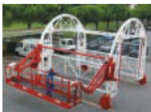
(Left) Safi's TST-500 CE has been developed for the final stages of tunnelling applications.
