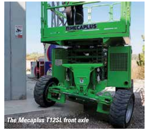
The Mecaplus T12SL can level by up to 12.3 degrees end to end to cope with a ground differential of 454mm
