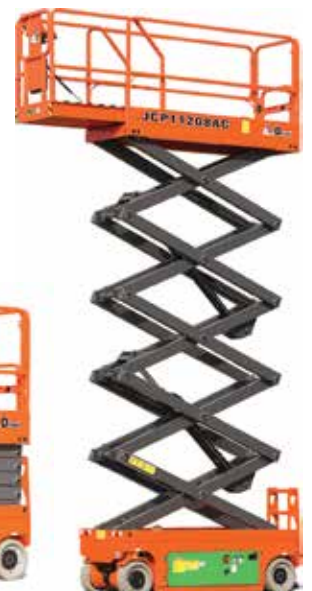
The 12 metre Dingli JCPT1208AC can drive at full height and has a 250kg capacity
