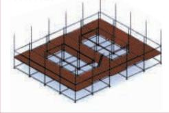
proceeds – often with those boards overlapping at the ends and unsupported between ledgers, making them bouncy and unsafe. SGB has taken the safe erection principles of SG4:00 and developed them to provide scaffolders with a safe method of erecting bird cage scaffolds.
