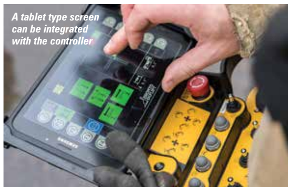
The basic controller weighs 2kg and can carry out all machine functions
