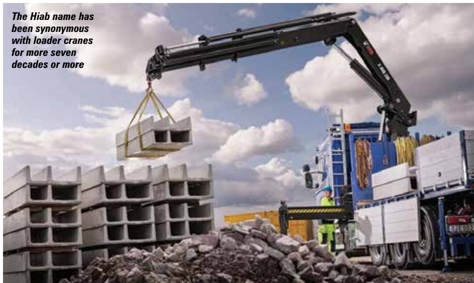
The electric/hybrid Hiab wspr crane
